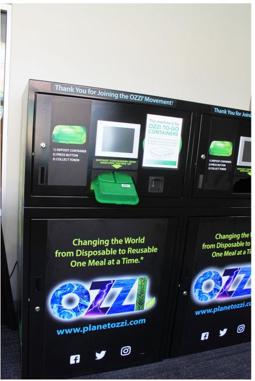
Kent State University Eastway Dining Hall utilizes PlanetOZZI O2GO containers and container return systems. Empty O2GO containers can be returned to the PlanetOZZI system. PlanetOZZI system machines read the barcode on the containers and then prompts users to hut a button to get a coin in exchange. When a user has a coin they can take it to the desk attendant to receive a new container. Photo by Leah Graham
