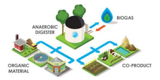
Anaerobic digestion, which is relatively new to Connecticut, is a biological process that breaks down food waste and other materials into combustible methane gas.
